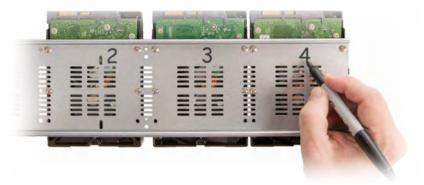
Line up the holes in the mounting bar over the drives, then use four of the screws supplied with the recorder to secure each drive in place.
