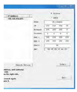
Check the camera data at the top of the right column. It may be that the camera is set to a static IP, and this static IP address is incompatible with your system's subnet address (see the example at left).
