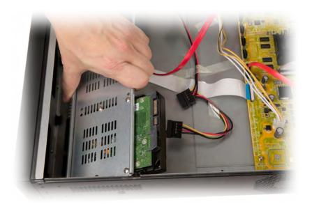
Remove the mounting bar by lifting the rear side, then pulling the entire bar away from the front of the recorder.
