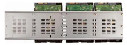
Lay the new hard drives to be installed side by side on a flat surface with the power and SATA ports facing the same direction and the circuit board on top.
